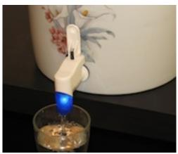
UV Aquastar has designed simple, affordable devices that treat water with ultra-violet light, killing pathogens and enabling people to take control of supplying their own safe drinking water. A mobile (bottle or stirrer) and a spigot integrated into water dispensers can be powered by battery, solar panel or grid.
